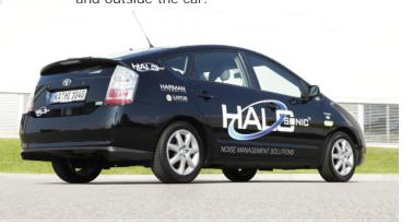
Using the same design principles deployed in high-end consumer and professional audio, the HARMAN HALOSonic controller synthesizes traditional engine sounds in direct correlation to vehicle speed. These are projected from the front of the car to alert nearby pedestrians through high-fidelity speakers, and may also be experienced inside the car at the driver's option.
